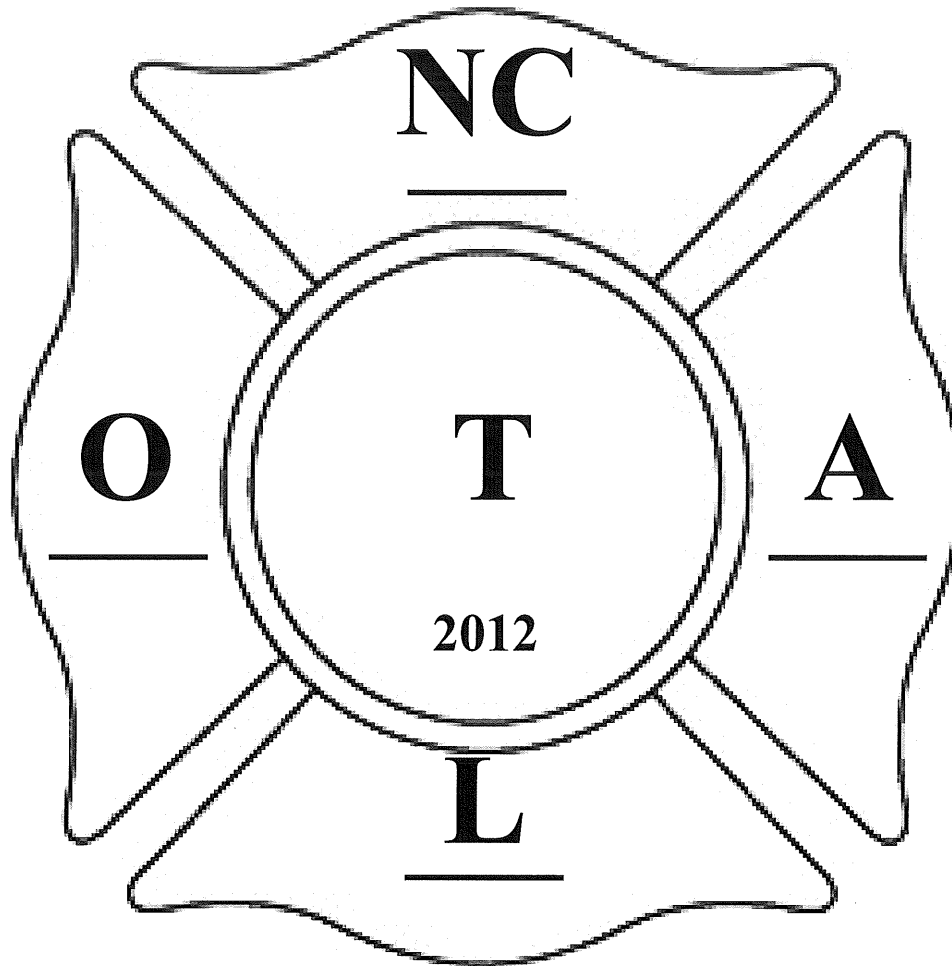
Portland Fire Fighter Safety Building Marking System Reflective white background
