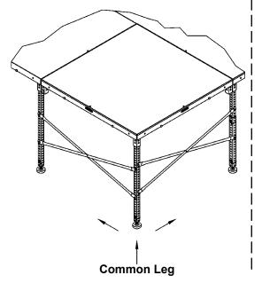
E. Multi-Stage should be braced every 2-3 decks as shown when bracing is required. (Note the common leg bracing method is shown below.)
