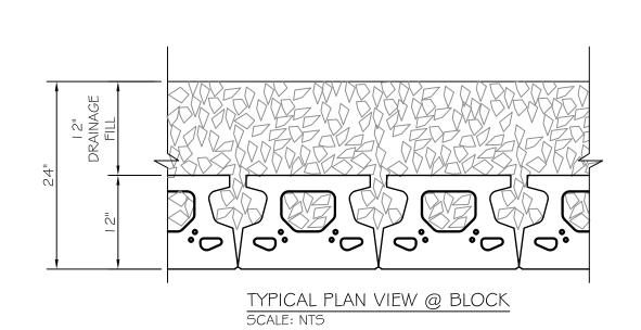
CRUSHED STONE UNIT COMPACT WITH HAND OPERATED PLATE COMPACTOR FILL ALL VOIDS INCLUDING PIN HOLES AFTER BLOCKS ARE ALIGNED. ALIGN EACH BLOCK COURSE PRIOR TO PLACING ADDITIONAL COURSE.
