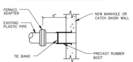
METHOD 1- EXISTING PIPE INTO NEW STRUCTURE
