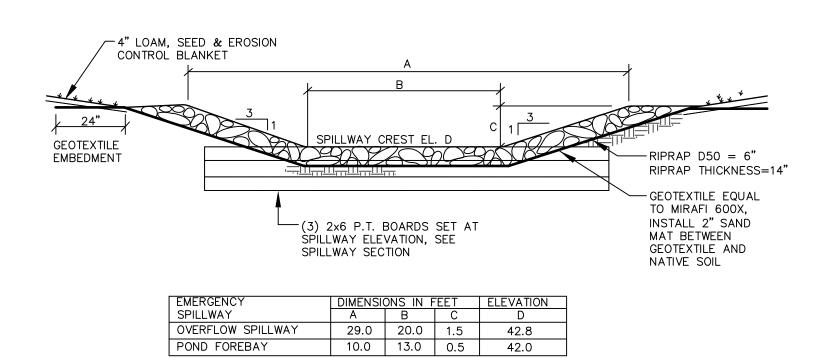
EMERGENCY/ FOREBAY SPILLWAY CROSS-SECTION NOT TO SCALE
