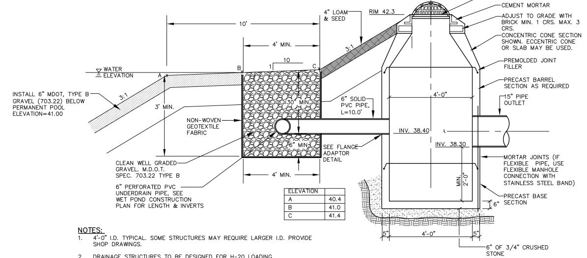
2. DRAINAGE STRUCTURES TO BE DESIGNED FOR H-20 LOADING.
