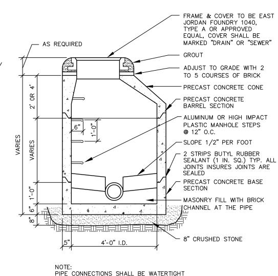
PRECAST DRAIN MANHOLE NOT TO SCALE
