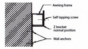
These are existing awning frames that are made from 1" square galvanized steel tubing. All welded construction. We will be recovering them with new fabric and installing them at the new location at 508 Riverside.
