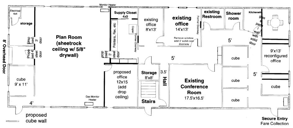
\_\_\_\_ 2"x4" partition wall to be removed
