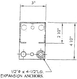
3" MINIMUM EMBEDMENT INTO -LOOR SLAB (I PER FOOTPLATE.)
