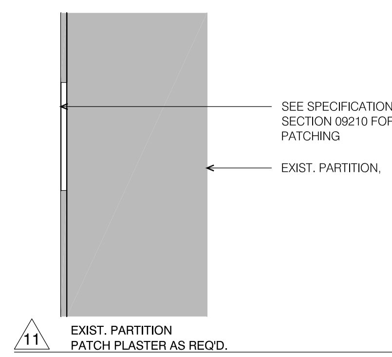
11 EXIST. PARTITION PATCH PLASTER AS REQD.
