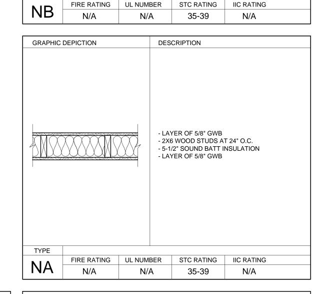
1.) REFER TO STRUCTURAL DRAWINGS FOR STUD SIZE AND SPACING
