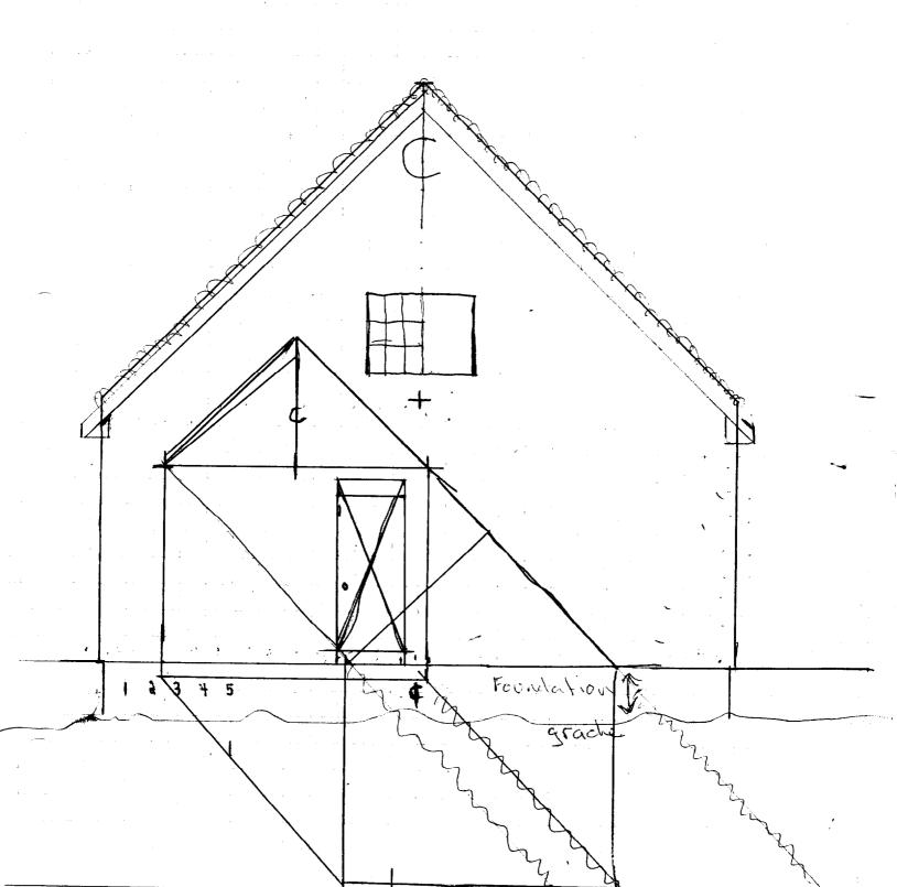
10X12 PT Deck and wrailing Front Leck \* notes 10x12' deck will be Framed WI 2X8 PT and 5/4 PT decking anchored to Entryroom, carried by 2x8 carring beam (double) on HX4 posts w/ 8" Sonotubes for foundation \* Railing Profile 36" Taltur/less NOTE is than 4"Spaceing Tairs of ballusters will haute and HX4 posts 4 on ¢ 711. 515e 2X8 PT Framing 12" Tread double 2x8 carring beam (PT) K 4X4 POSTS <- 8" Sonotubes" 4 deep \* Scale: 12"=1
