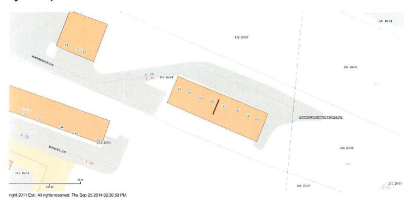
The wall was put up between unit #67 (New England Carpenters Training Fund Unit) and Unit #65 to separate the units. The wall does not go the entire length of the building because there was already a wall that separated the units on the ends; please see the A1ExistingWall.pdf which shows the section of wall that was added which is 17' 4" long.
