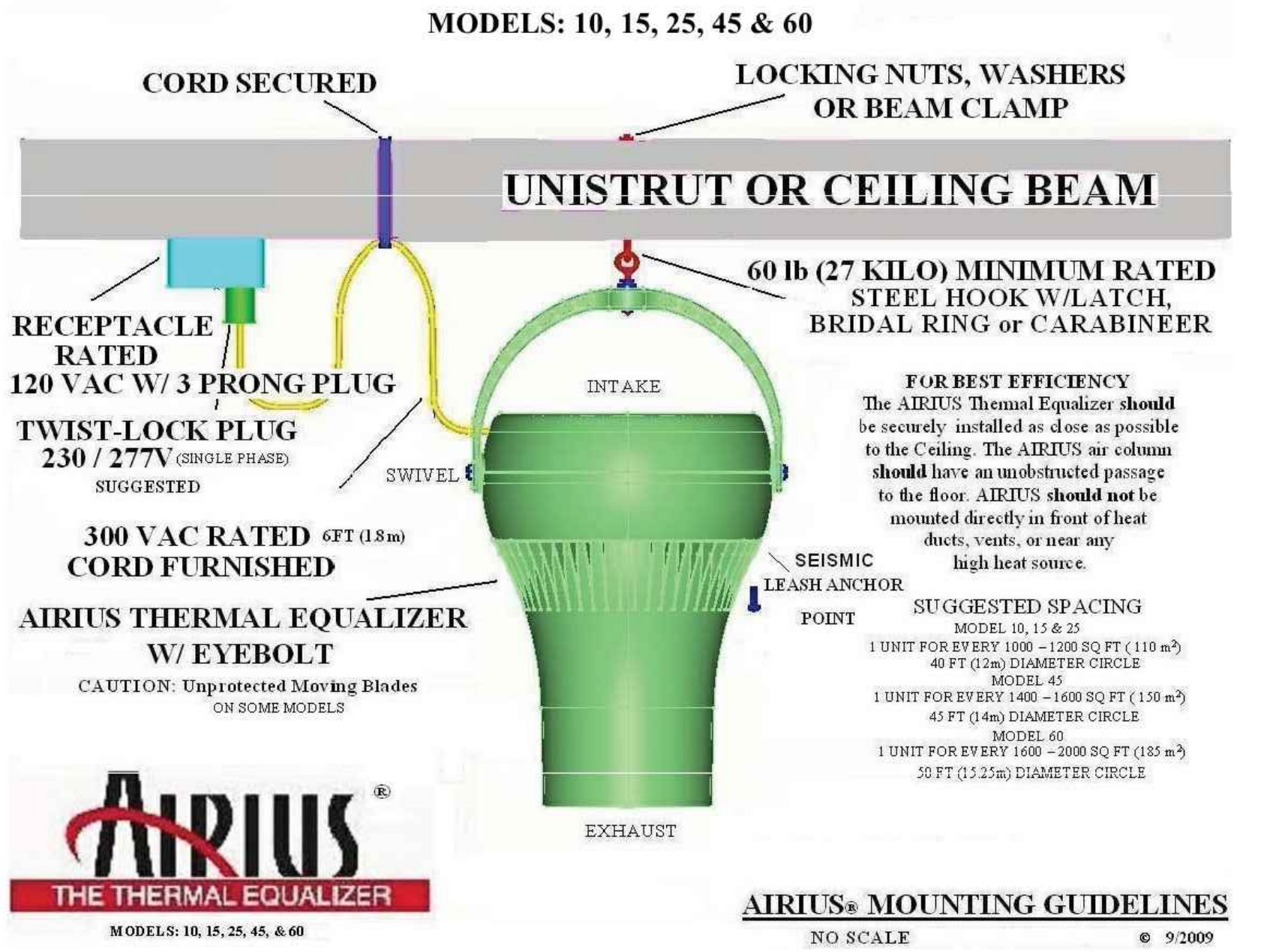
4 DESTRATIFICATION FAN INSTALLATION MOUNT TO JOIST AS HIGH AS POSSIBLE NOT TO SCALE
