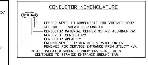
SINGLE LINE FEEDER SCHEDULE 60-4C (4)#4 AWG CU & (1)#10 AWG CU GND. IN 1-1/4" CDNDUIT FEEDER SCHEDULE GENERAL NOTES • FEEDERS DENOTED BY A "\*" HAVE BEEN OVERSIZED TO COMPENSATE FOR VOLTAGE DROP. "CU" = COPPER CONDUCTOR • "AL" = ALUMINUM CONDUCTOR ALL CONDUCTOR AND CONDUIT SIZES SHOWN ARE MINIMUM REQUIREMENTS, INCREASE SIZES AS NEEDED TO ACCOMMODATE VOLTAGE DROP, DE-RATING, SITE CONDITIONS, AND MEANS AND METHODS USED FOR INSTALLATION OF FEEDERS.
