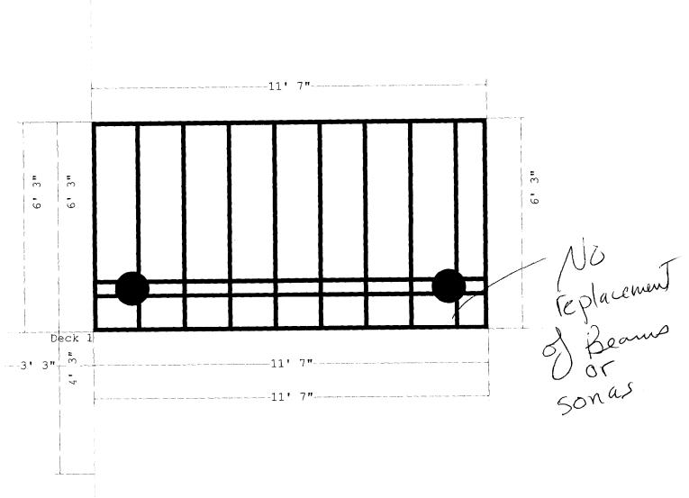
Joist Spacing = 16 in. o.c. Baluster Spacing = 3 3/4"
