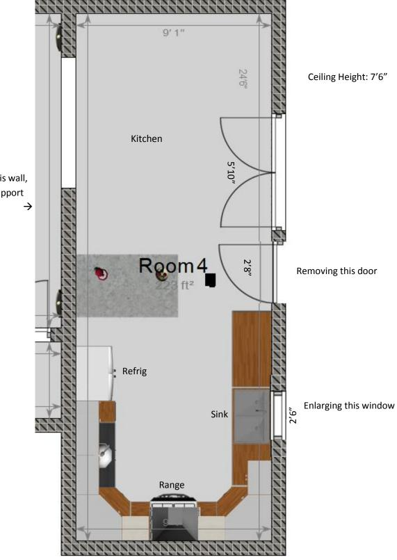
Removing part of this wall, and replacing the support beam in ceiling
