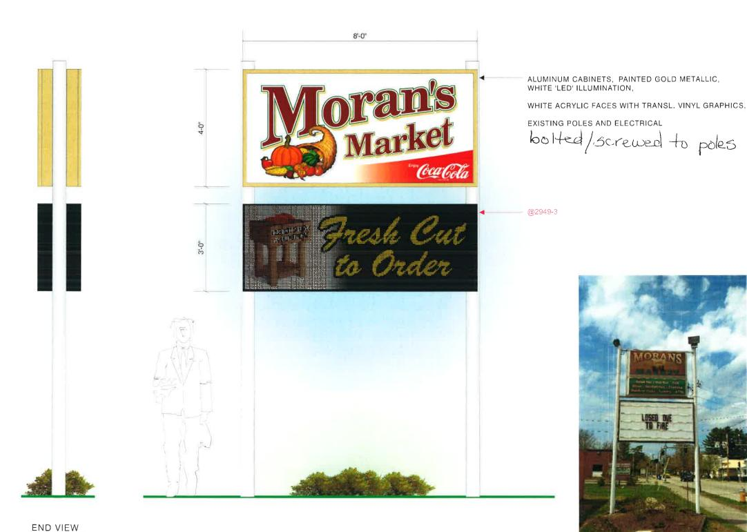
D/F IN. ILLUM. SIGN - EXISTING PYLON STRUCTURE SCALE: 1/2"=1'-0" (1) REQUIRED
