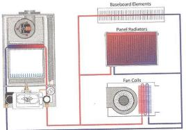
The Solenne Classic Boiler is perfectly suited for heat distribution systems designed to utilize high temperature water.
