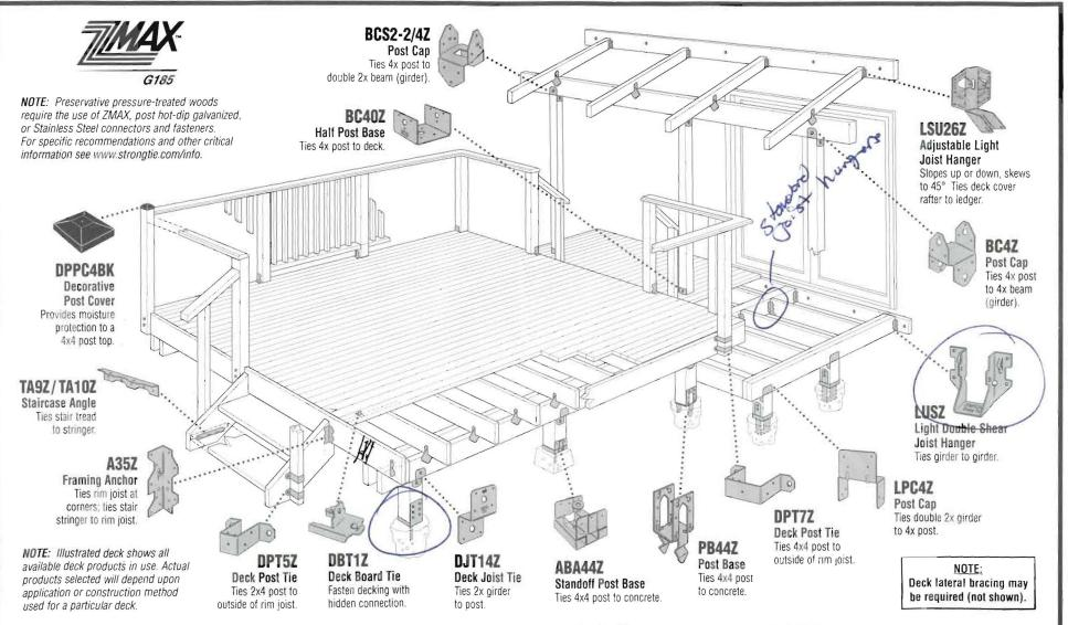
A Complete Connector System for Deck Construction • Install Deck Boards with NO Surface Nailing!
