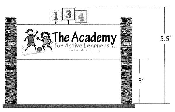
Sign is 2'h x 6' wide - mounted to 2" x 4" framing and 6" x 6" wooden posts. posts are covered with faux stone covers from home depot post holes will be 3' deep with be 8" sonotube filled with concrete
