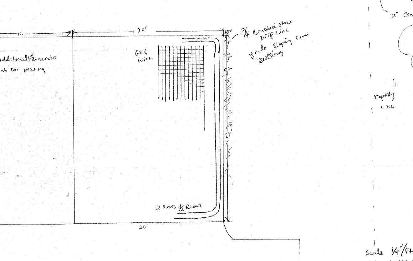
Slab side View RuiForced 4" stab wire Remforced grade 12" Compacted gravel fill 1/2" Proit@6'oc. Embedded into slab and CMU perimoter and CMU perimoter block with Extension property Line
