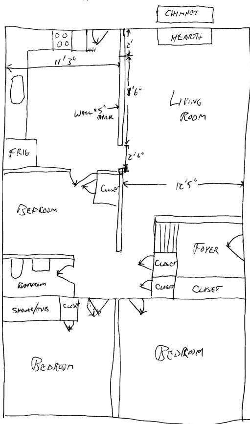
FLOOR AND CEILING JOISTS RUN PERPENDICULAR TO KITCHEN WALL
