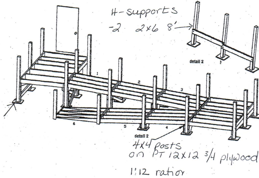
Note: The same options for transition to the ground are used for this design. Guardrail/handrail options are also the same except the inside guardrail on the lower portion of the ramp will be attached to the center 4x4's. Between modules 3 & 4 some 2x2x30" spindles will need to be screwed in place from inside the ramp.
