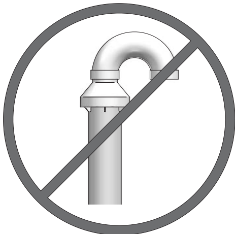
Figure 5-5 Do Not Install U-Bend to Rain Cap
