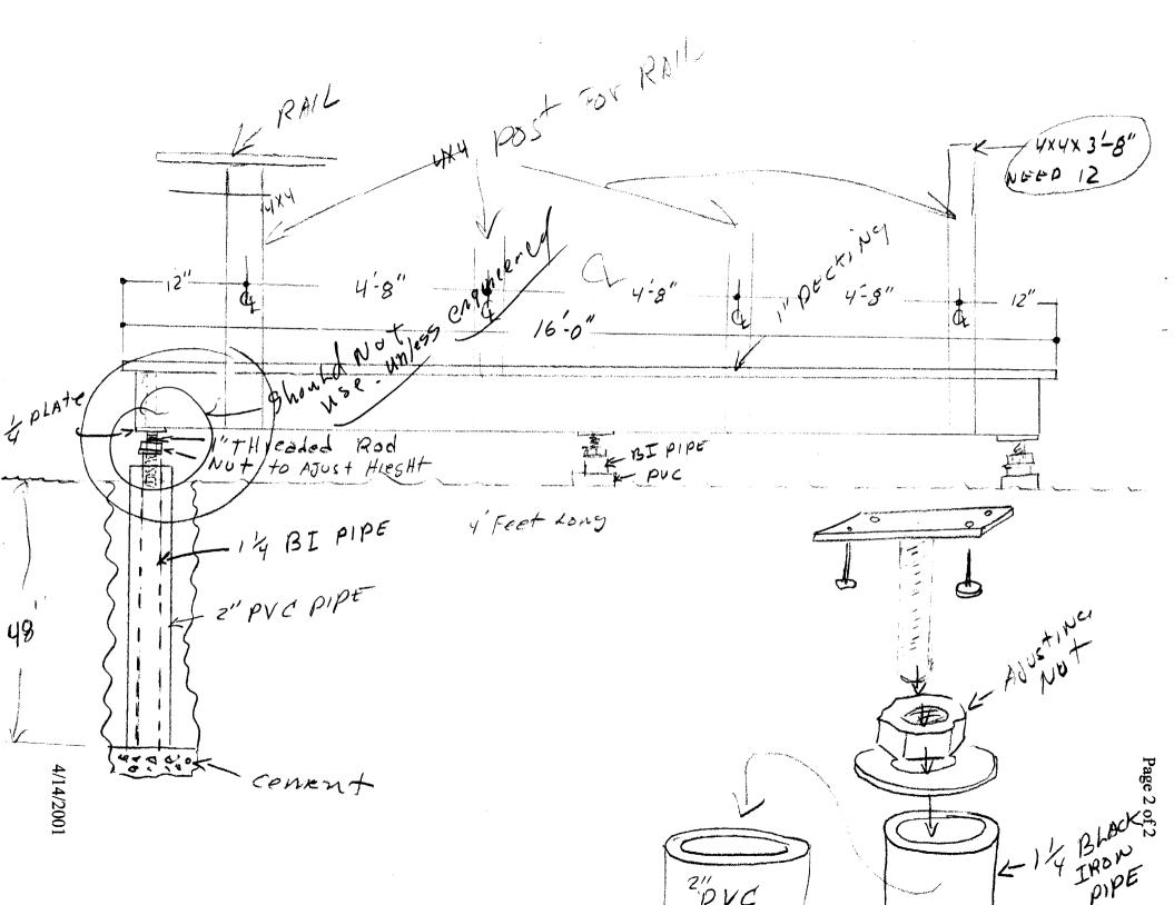
4x4x8' For RAIL Post L top RAILS SIDE RAILS Guand xa. C. 1021.0 treated lumber raming, joists etc. Frotings 4' deep (3)
