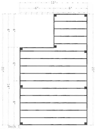
Joist Spacing = 16 il" o.c.5' ll" - - - 6' - - - Baluster Spacing = 3 3/4"
