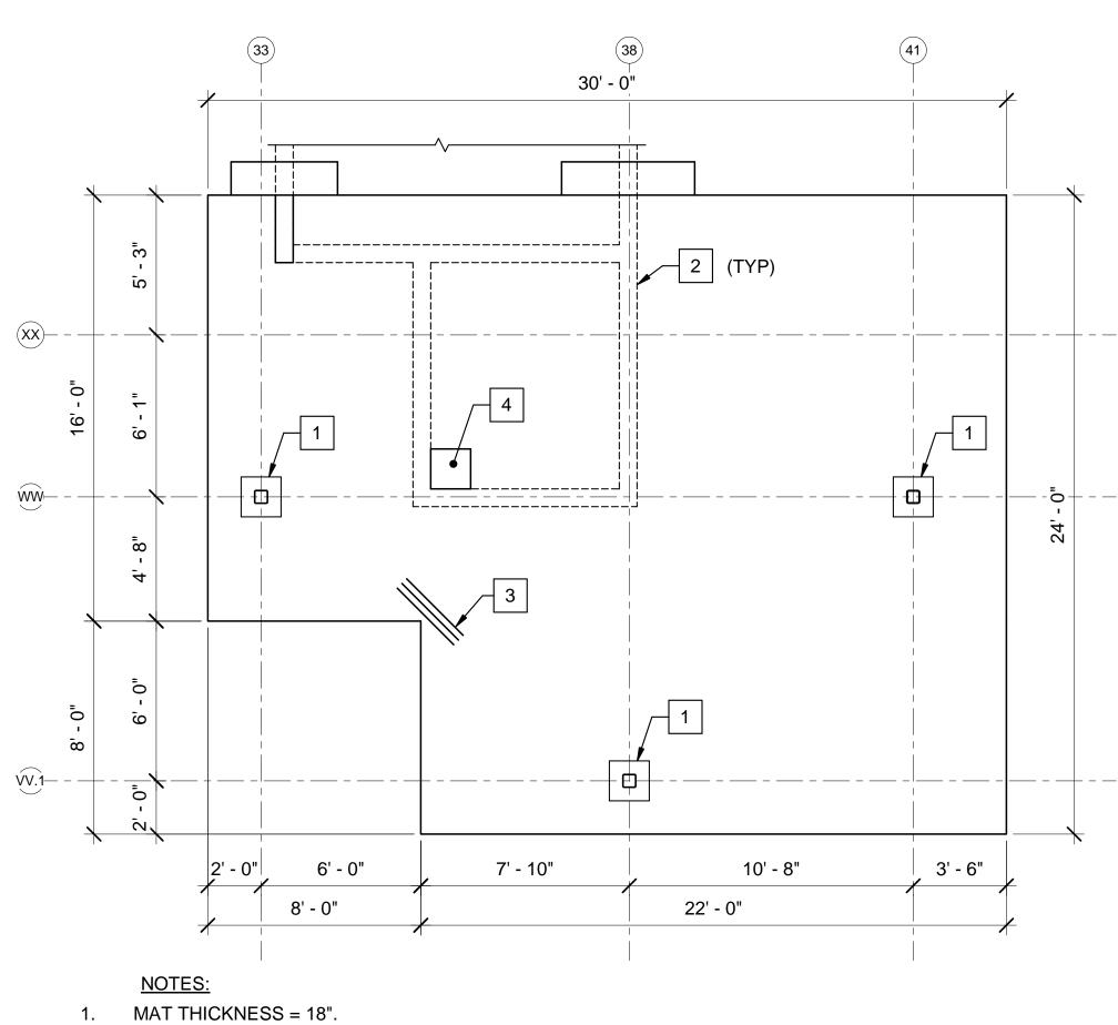
2. REINFORCING: EAST-WEST = #6'S AT 15" OC TOP AND BOTTOM. NORTH-SOUTH = #6'S AT 9" OC TOP AND BOTTOM.
