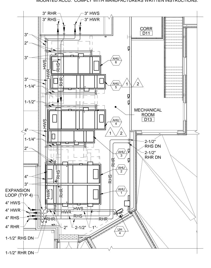
SECOND FLOOR MECH ROOM D13 PIPING PART PLAN
