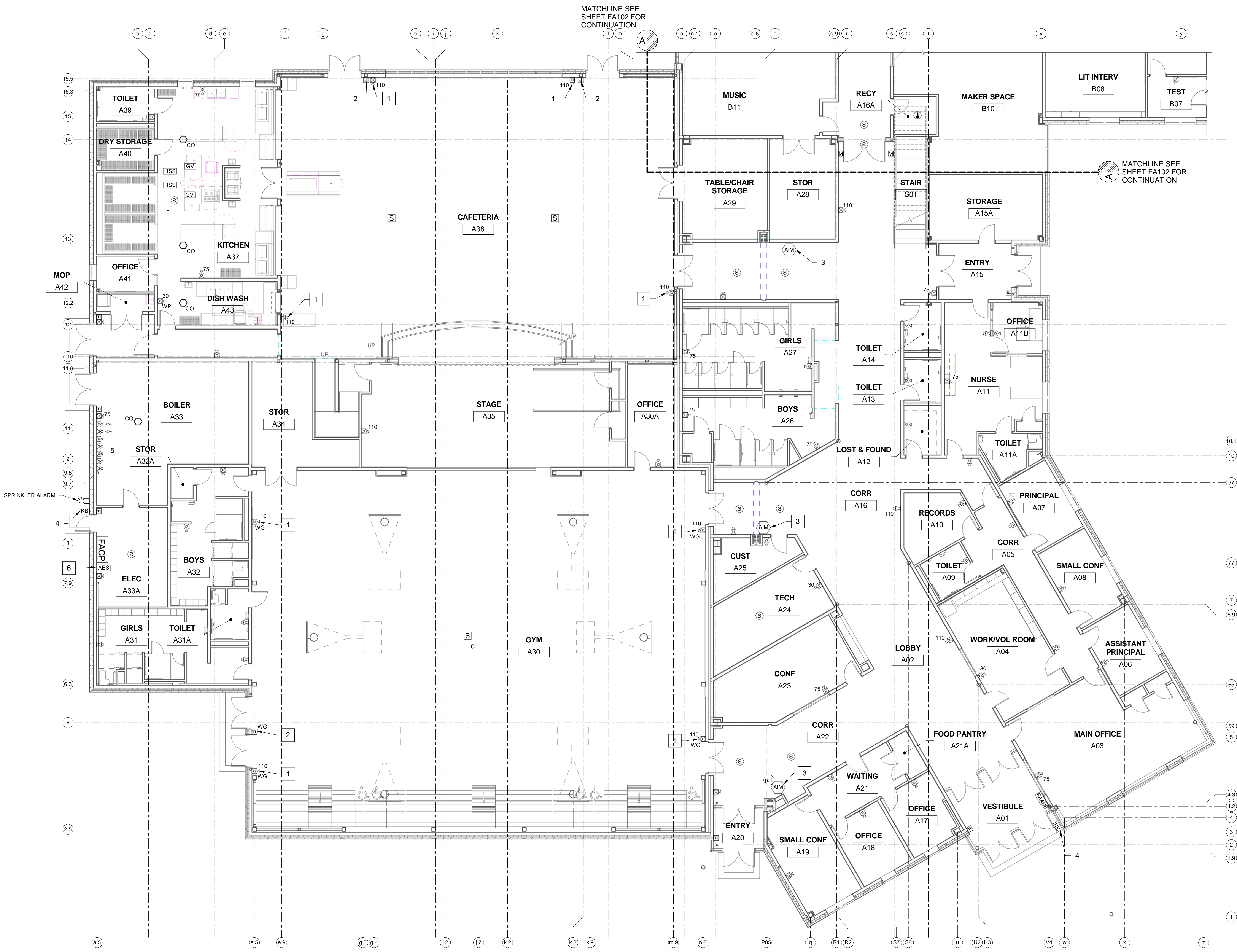
1 FIRST FLOOR FIRE ALARM PART PLAN A FA101 SCALE: 1/8" = 1'-0"
