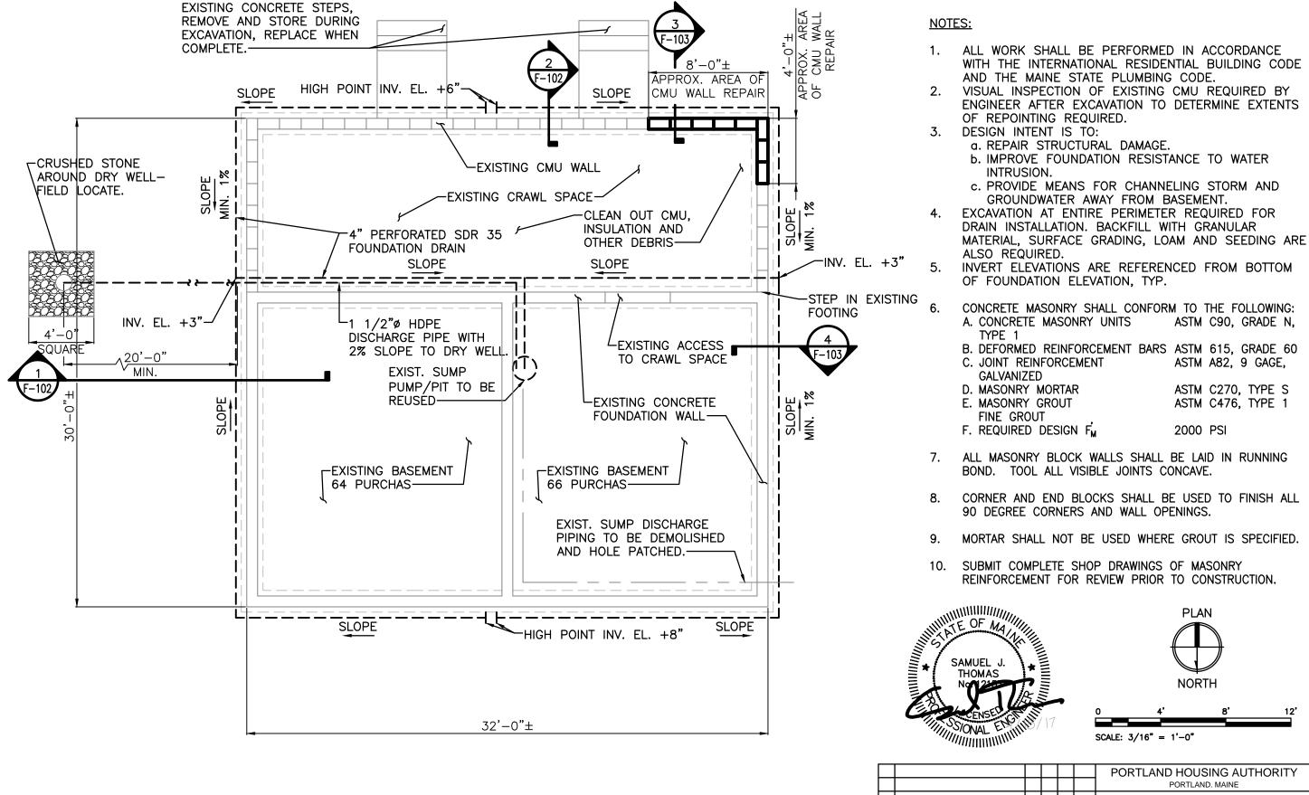
FOUNDATION AND DRAINAGE REPAIR PLAN
