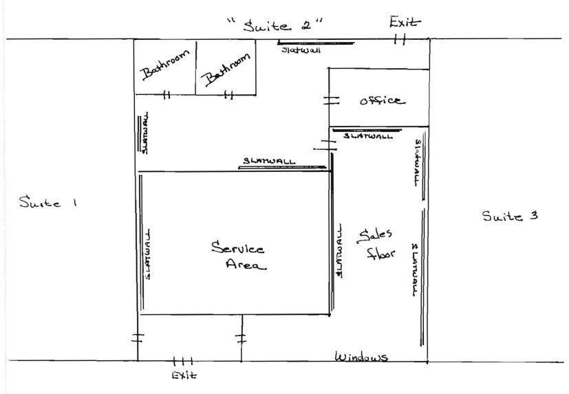
I latural is a heavy paneling used to hold display brackets for retail Sales. We used 20 screws Per sheet - Self tapping and sheetrock screws -This slaturall has a "C" Rating - The building is a Steal Frame building Building Layout is the Same.
