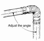
The lengths of the air intake hose and the exhaust pipe must be the same in order for the appliance to operate properly. The hose can be cut to the required lengh. Deburr all rough edges. Do not cut the hose attached to the appliance.
