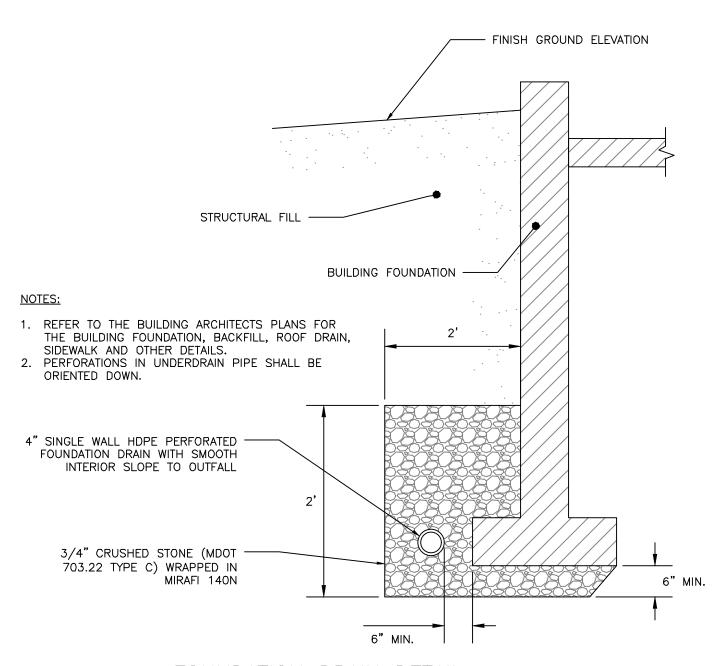
FOUNDATION DRAIN DETAIL NOT TO SCALE
