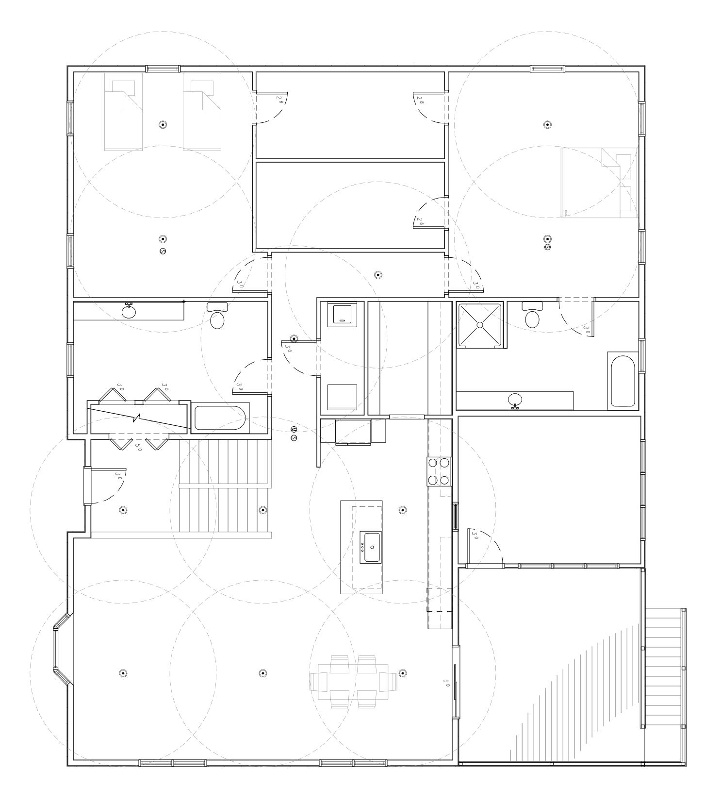
1 FIRST FLOOR SPRINKLER PLAN A10 SCALE: 1/4" = 1'-0"
