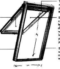
Top sash opens for maximum ventilation, pivoting inward for easy cleaning
