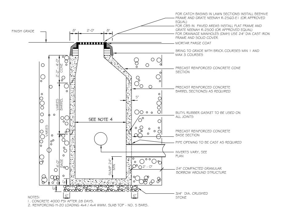
PRECAST CONCRETE CATCH BASIN / DRAINAGE MANHOLE (ONSITE)
