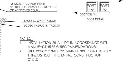
PREFABRICATED SILT FENCE NOT TO SCALE
