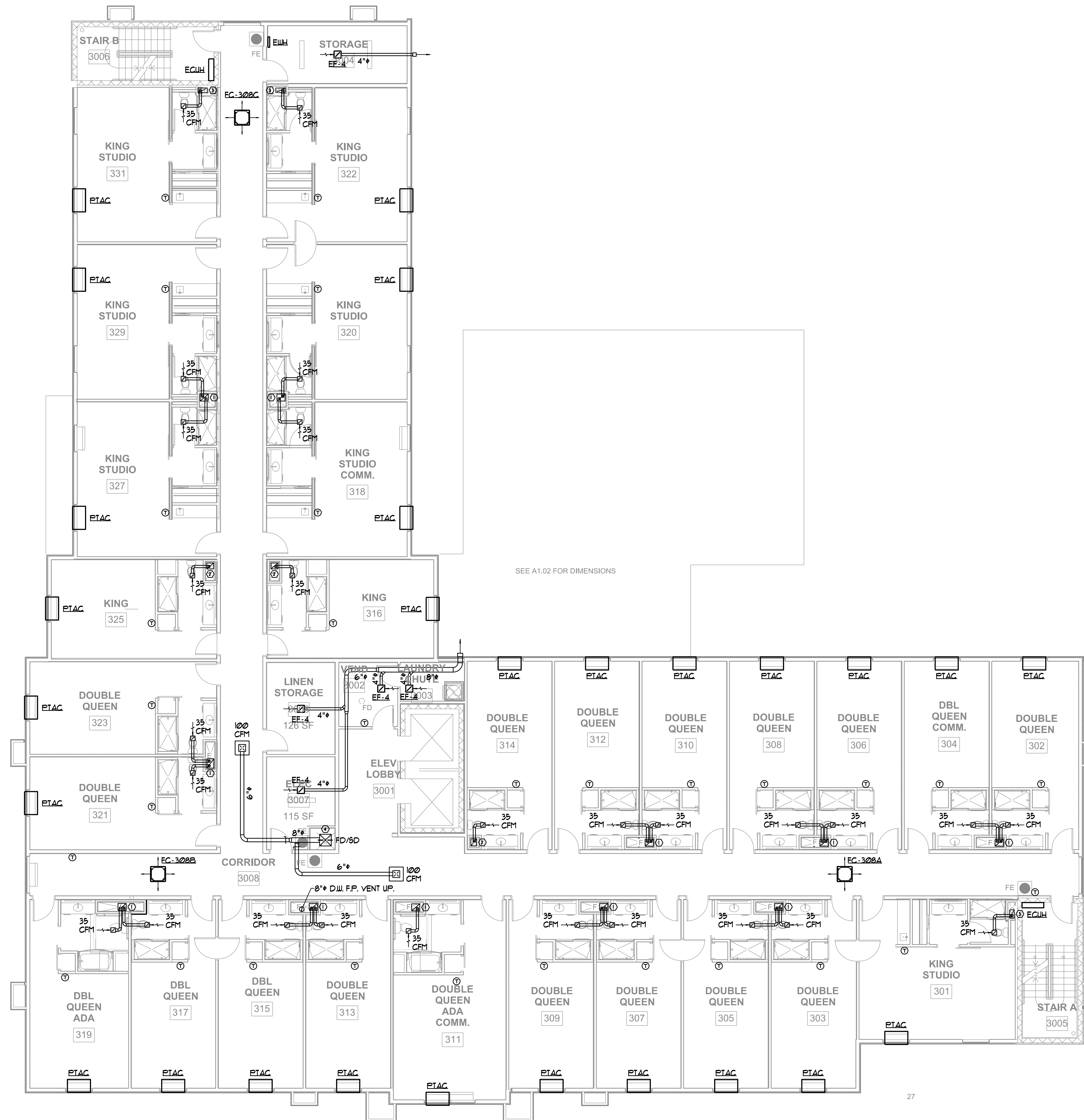
THIRD FLOOR MECHANICAL PLAN SCALE - 1/8" = 1'-0"
