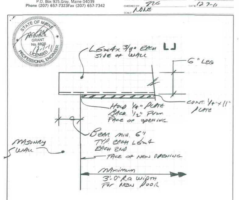
ELEVATION VIEW: TYPICA BEARING (Never TO 5K-1)
