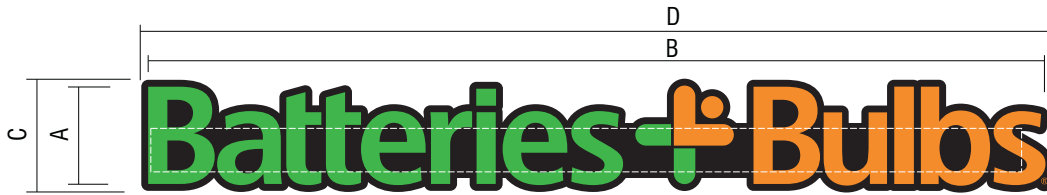
Lineal Channel Letter Front Detail - Custom Raceway Mounted (RW) Not To Scale
