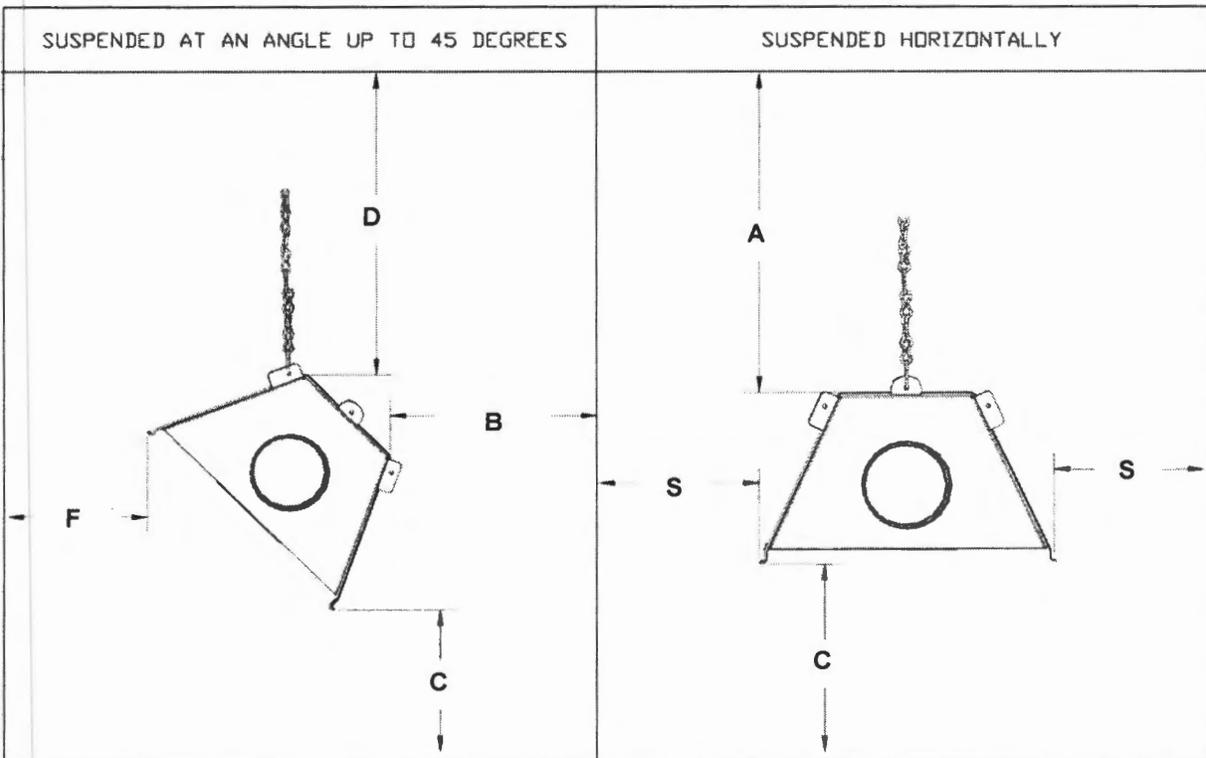
The clearance to combustible material represents the minimum distance that must be maintained between heater and a nearby combustible surface. The stated clearance to combustibles represents a surface temperature of 90°F (50°C) above room temperature. Some materials such as awnings or plastic may require higher clearances. It is the installer's responsibility to ensure that building materials with a low heat tolerance which may degrade at lower temperature are protected to prevent degradation.
