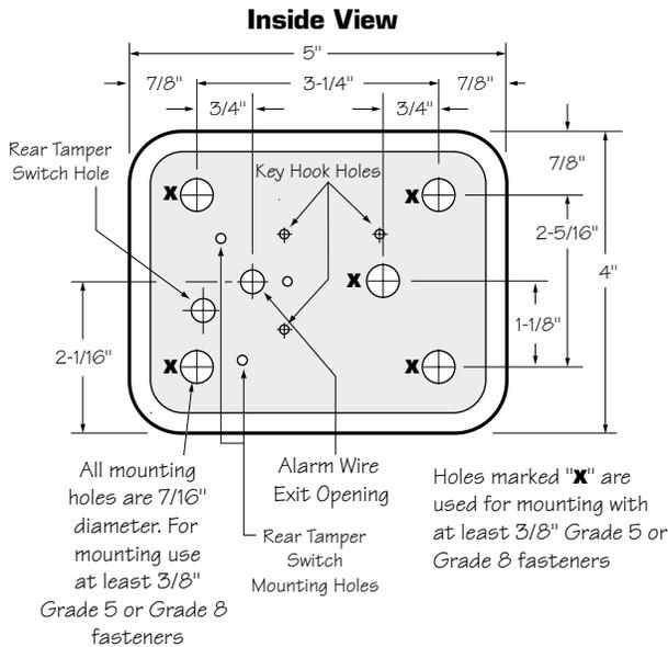
**Attention: KNOX-BOX® is a very strong device that MUST be mounted properly to ensure maximum security and resist physical attack.**
