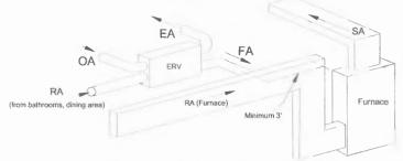
Note: ERV Blower may be operated separate from Furnace Blower.
