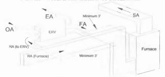
Note: The Furnace Blower must be operated any time the ERV is operated.
