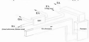
Note: ERV Blower may be operated separate from Furnace Blower \*Use caution to introduce FA at low velocity and where good mixing will occur to minimize discomfort from drafts.
