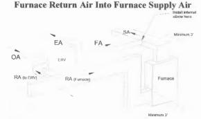
Note: ERV Blower may be operated separate from Furnace Blower.
