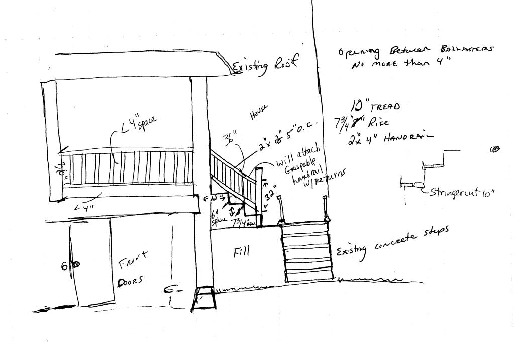
Est. cost of Tob \$1,000.00) 32 Lucas str. HAND RAILS 2x2 5"o.c. 42" High Tom & KAthy Chadbourne 16' x 641/2" Porch (Existing Roof) legge Attached to House 5 134 oc. W 3" LAY BOLLS GAKY 1/2 Existing Roof the Beam Existing is 5'13/1" 0.C. 4" × 6" Fax Heades 4x 10" Header Set BACK From street 21'71/2" 424 FRON+ brackett TO PIET 4' FROST PIER (PRECOST) Reinbroad 10"
