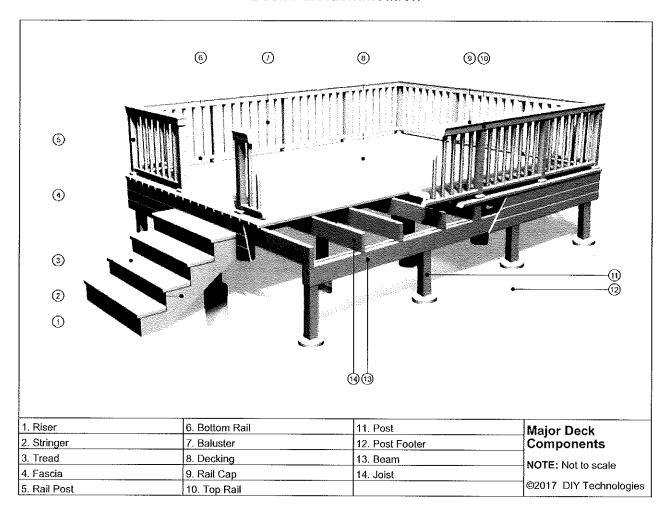
Baluster The vertical pieces of a railing spaced at regular intervals between posts. Beam A horizontal framing piece, which rests on posts and supports joists.
