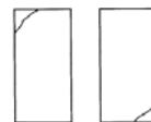
Type 5 Side fractures at top or bottom (occur commonly with unbonded caps)
