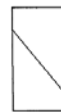
Type 4 Diagonal fracture with no cracking through ends; tap with hammer to distinguish from Type 1
