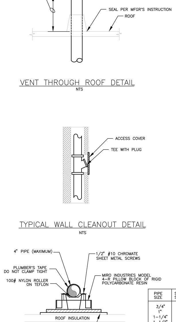
ROOF PIPING SUPPORT DETAIL
