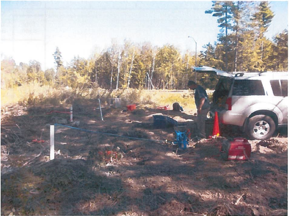
Photograph showing crosshole seismic testing setup. View to the northeast. The downhole source is located in borehole GB-102 (white casting with blue air hose in foreground, bottom left). The downhole geophone is located in borehole GB-101 (white casting with pink ribbon, center left). Both seismic source and geophone are connected via cables (not seen) to the seismograph, located in the back of the truck. The partially completed access road to the site is in the background.
