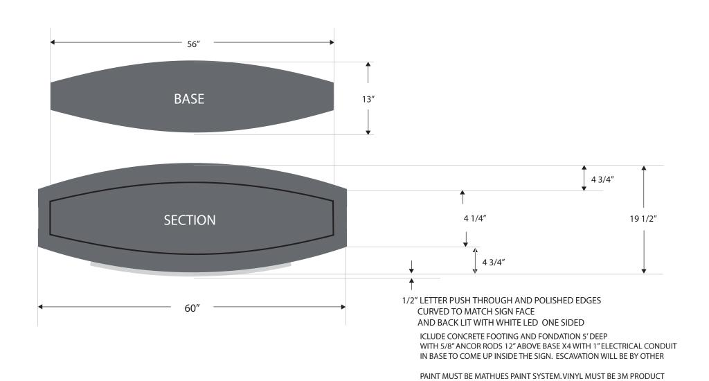
SIGN IS CONSTRUCTED OF 1/8"THICK ALUMINUM WITH ALUMINUM RIB STRUCTURE INSIDE
