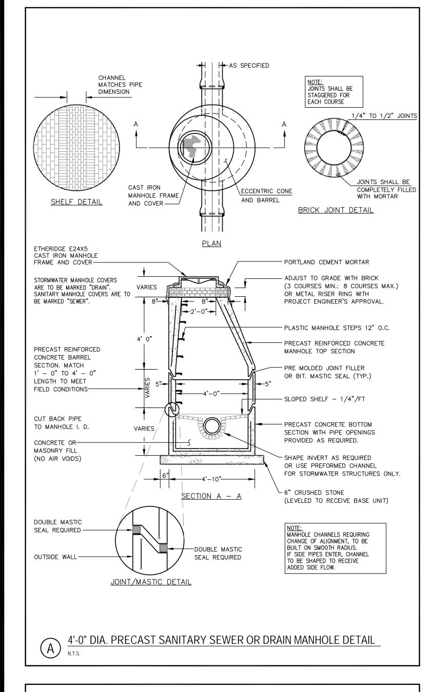
BRICK MASONRY CHANNEL, CARRY VERTICAL FROM SPRING LINE TO CROWN
